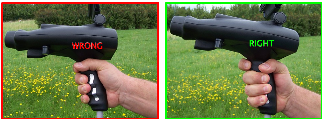
Figure 6.2: Contact between operators hand and the electrodes
