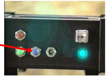
Battery Level Test Button
