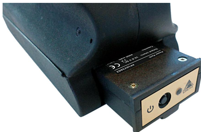
Figure 5.3: Placing the Power Pack into the telescopic rod assembly
