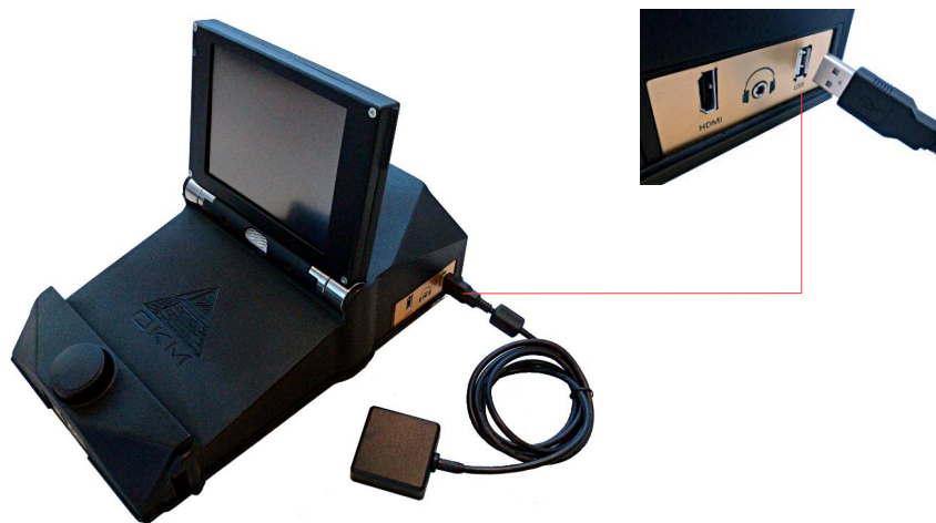
Figure 5.5: Connecting the external GPS receiver
